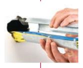
Ready™ Sleeve convenience for existing cable installations. Split sleeve and two-piece wall plates allow sleeve to be assembled around cables and locked into the wall or floor. Available in 1" (33 mm OD), 2" (60 mm OD), and 4" (114 mm OD) sizes.
