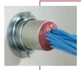
A complete code compliant firestop sleeve assembly for new cable installations. Includes all mounting hardware and internal and external firestop sealing materials. Available in 1" (33 mm OD), 2" (60 mm OD), and 4" (114 mm OD) sizes with standard or large escutcheon plates.
